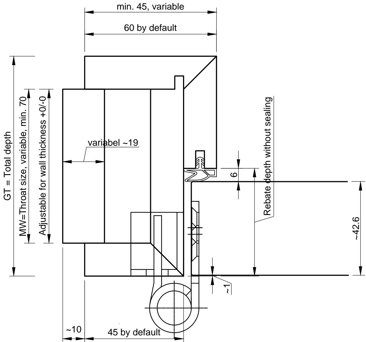
Face width varies based on hinge type and mounting conditions
