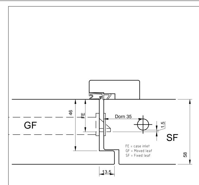
Rebate retracting bolt, locks automatically in upper and lower positions
